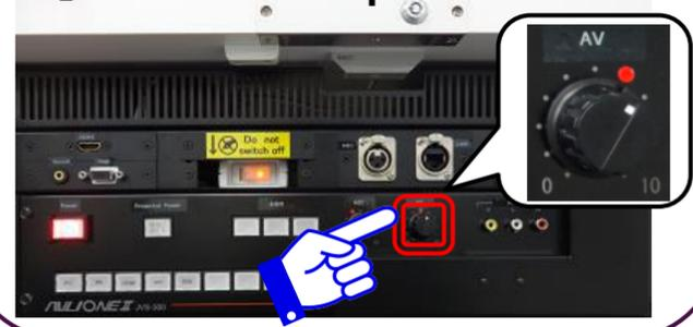
**6** to adjust the volume for wireless microphone, use [MIC] volume knob. 「●」is the standard position.
