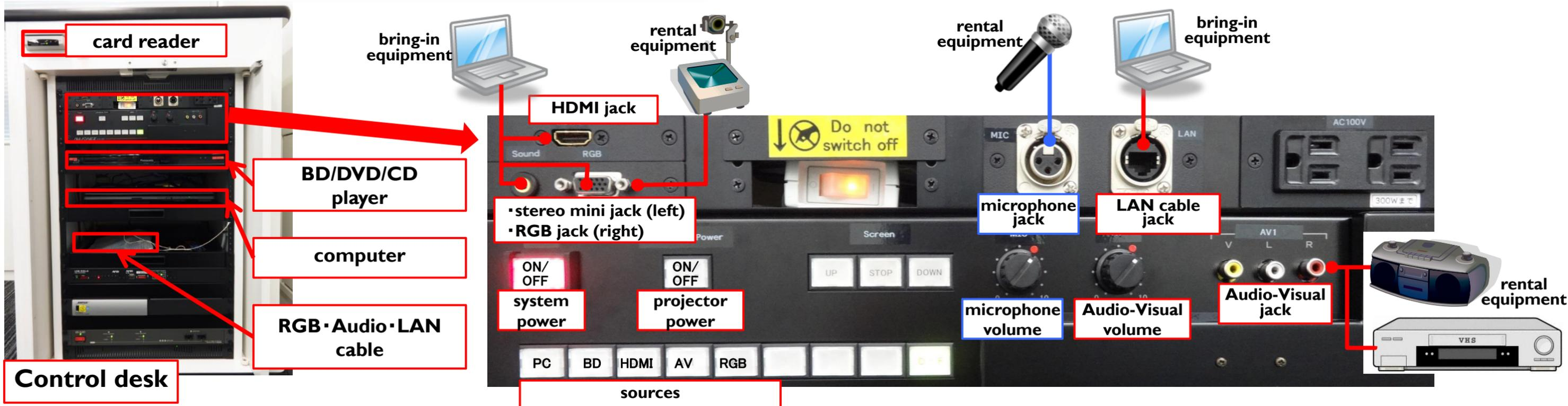
**1** swipe the ID[S] card through the card reader to open the cabinet and turn on the system power.
