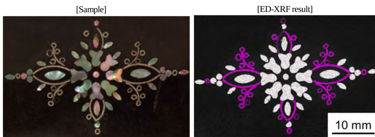
Figure 2 Surface mapping by ED-XRF (Gray: Pb, White: Ca)
