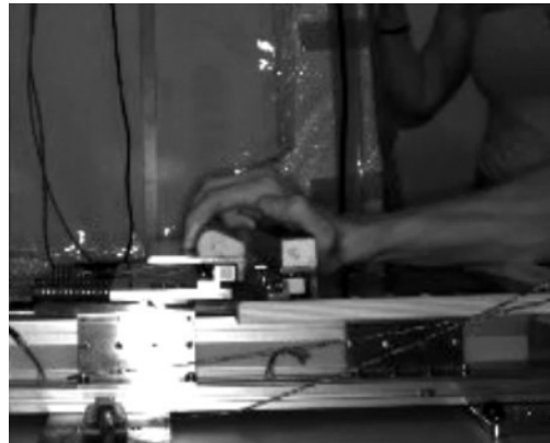
Figure 2. Left: Hangboard condition with the finger hold fixed and the robot mounted vertically. Right: Robot condition with the robot fixed horizontally on a table and a palm rest to create a counter force.
