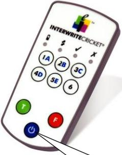
The image shows an Interwrite Cricket remote control. A callout box points to the power button at the bottom, labeled '電源ボタン'. The remote has several buttons labeled with letters and numbers: 1A, 2B, 3C, 4D, 5E, 6, and a power button.
