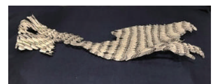
自動車内装材を一体型ハニカム構造で再現 (萩原一郎) Integrated Kirigami honeycomb structure reproducing a part of an automobile interior (HAGIWARA Ichiro)
